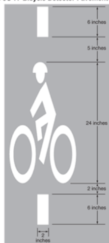
FIGURE 3--SIGNAL LOOP MARKING
